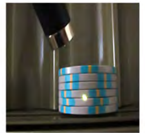
Detecting the chips in a stack or float tray
